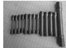
Fig. 1.b Round tension test specimens
