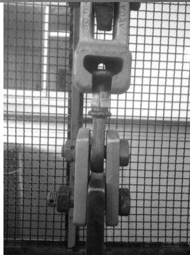
Fig. 9 Geometry test set up for ball tang
