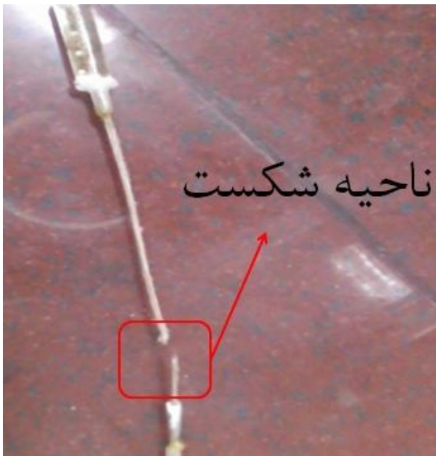
Fig. 3 Tensile Failure of impregnated jute composite
