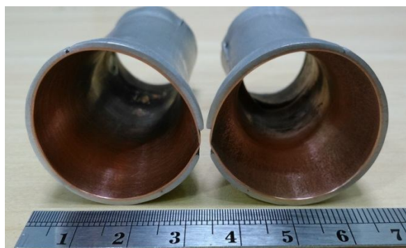
Fig. 9 two layers composite tubes of copper - aluminum after forming by HMGF process
