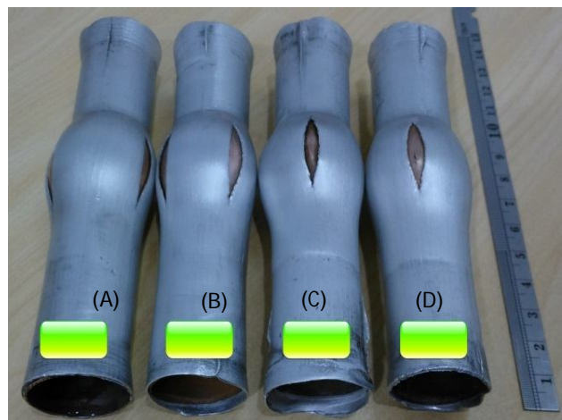
Fig. 13 Two layers samples formed by HMGF process at various conditions, A) Isothermal-570 ° C, B) gradient -570 ° C, C) Gradient -550 ° C, D) Isothermal -550 ° C
