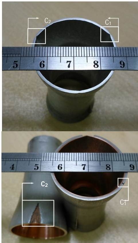
Fig. 20 Critical rupture zones C1 and C2 on the wall of single layer and two layer tubes by the process (HMGF)
