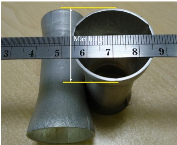
Fig. 14 A view of the maximum bulge of single layer aluminum tubes
