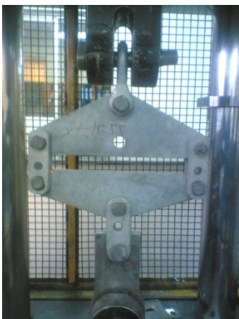
Fig. 7 Tension test set up of yoke plates
