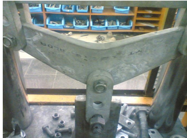
Fig. 8 Lateral buckling of yoke plate
