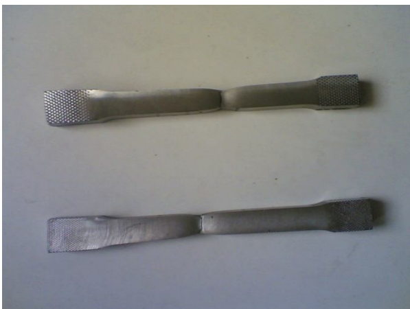
Fig. 6 Tension test specific from plate
