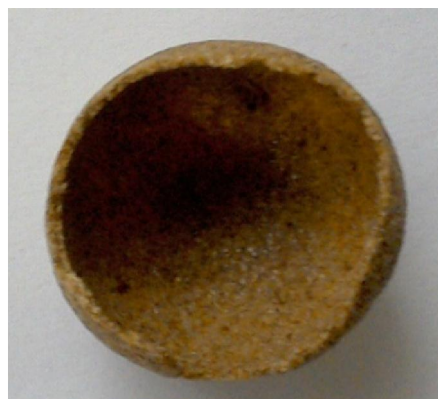
Fig. 6 Coating thickness 300-400 microns
