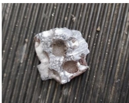
Fig. 10 Cavities created by lost foam casting
