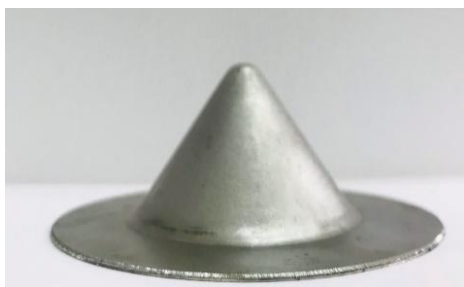
Fig. 13 A view of the sample produced in the first stage of the two-stage strategy
