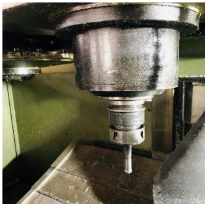
Fig. 3 The spherical head tool is placed on the tool holder and spindle of the machine
