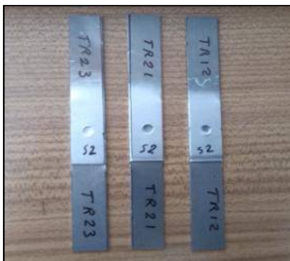
Fig 5 The samples prepared for tensile-shear test [10]
