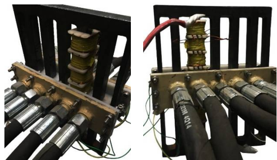
Fig. 5 Assembly view of constructed arrayed electromagnetic flowmeter when array number 2 is active
