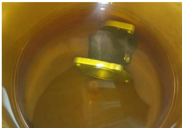
Fig. 27 Immersion in gasoline
