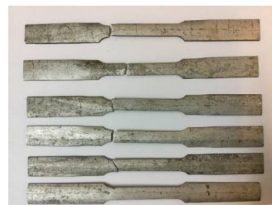
Fig. 2 Tensile test specimens for aluminum according to ASTM E8 standard
