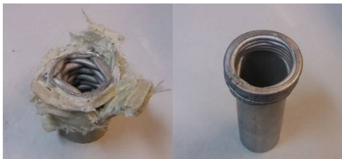
Fig. 7 Comparison of the hybrid tube crushing mode with aluminum tube
