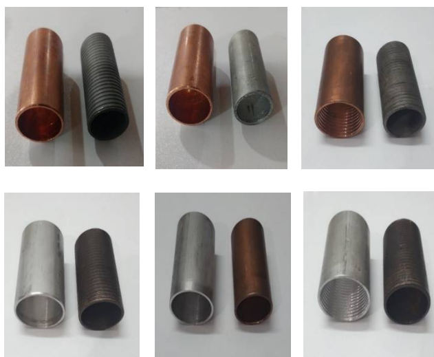
Fig. 3 Preparation of tube surfaces before assembly of bimetal tubes
