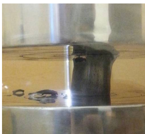
Fig. 11 Crushing test of aluminum shell and copper core bimetal tube with grooves in the aluminum and copper surfaces and at extrusion ratio of 60%
