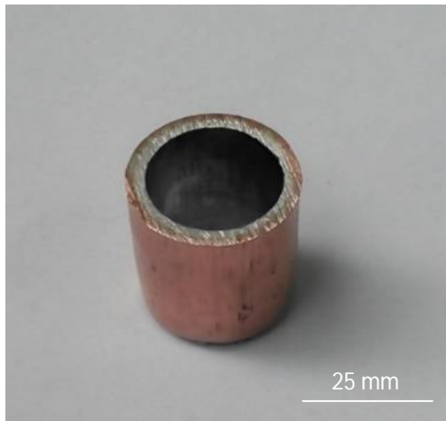
Fig. 1 Bimetal tube for forward extrusion
