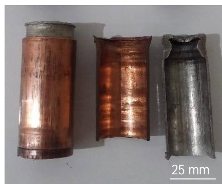
Fig. 5 Bimetal tube in extrusion ratio of 40 % with groove on tube surfaces
