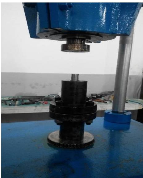
Fig. 4 Experimental Setup of die extrusion on press machine
